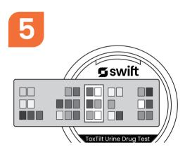
Read the adulteration test results at 3-5 mins using the colour card.
